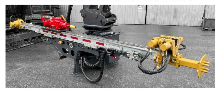
The TR-EX 1500 is a compact and high-performance excavator drill attachment designed for civil engineering works such as anchoring, soil nailing, casing, micropiles, and blast hole drilling.
